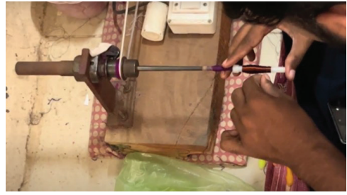
Figure 3: Copper wire on small bobbins called tillis
