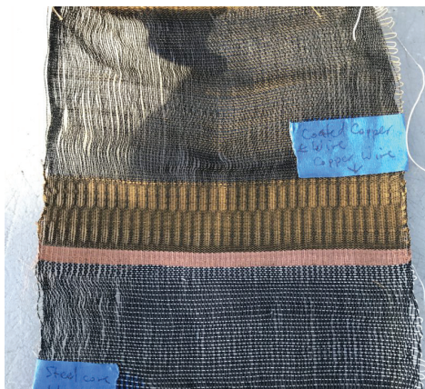
Figure 1: Coated copper wire, copper wire, steel-core thermoplastic woven cloth
